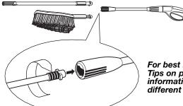
**Step 1** To install the high/low wand or wash brush simply insert into the spray wand extension. Press in against the spring tension and twist into the locked position. High/low wand must be set in the low pressure position to apply detergent.
